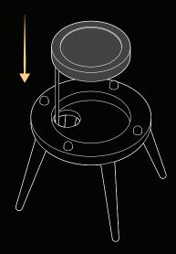
This fixture is designed for use with the included 3W LED disk only. Do not modify or replace with other light sources.
